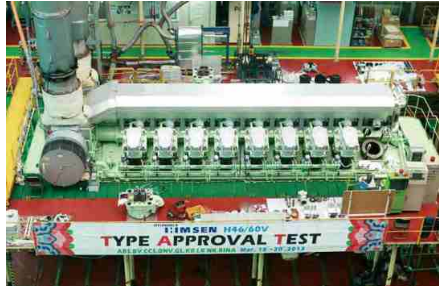
2013. 05 힘센엔진 8H46.60V Type Approval Test
